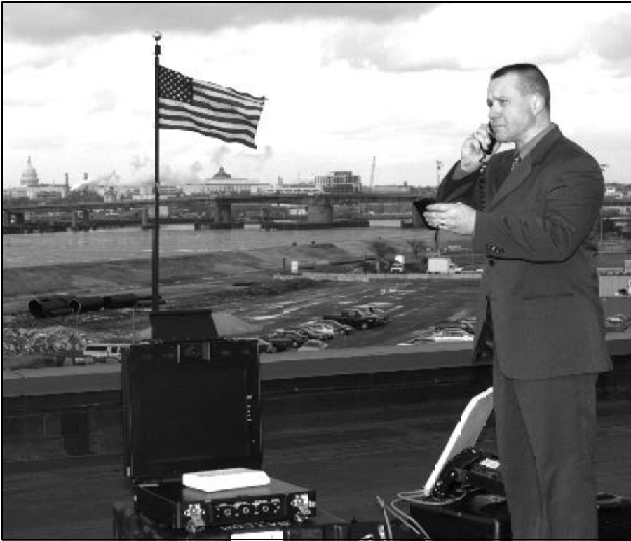
Figure 4. SFC Thomas White Jr., a 31P assigned to the Whitehouse Communications Agency's Directorate of Operations, tests voice and video teleconference capabilities on deployable INMARSAT terminal and secure satellite Video TeleConference equipment.
